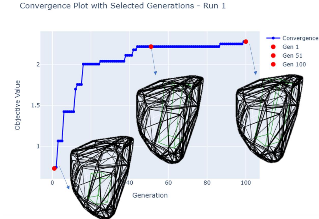
Fig.4. Snapshots of the cuboid (green) identification process at generations 1, 51 and 100 on the convergence plot for run 1, in the convexified granite rock
