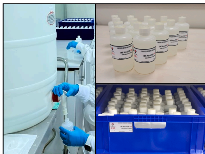
Fig. 2. Bottling of seawater in the TÜBİTAK UME ISO Class 6 Clean Chemistry Laboratory.
