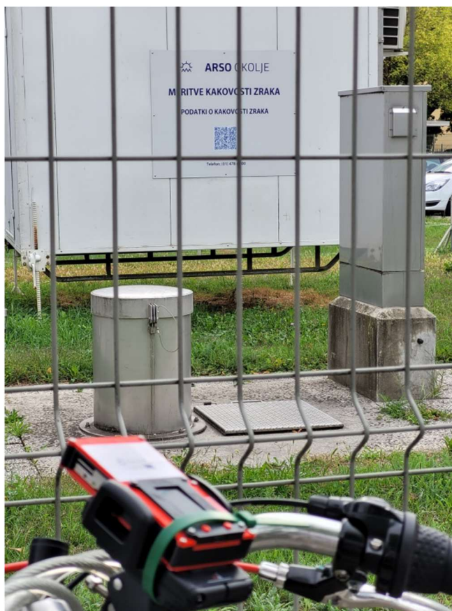
Figure 2. Co-location field assessment of LCS SPS30.
