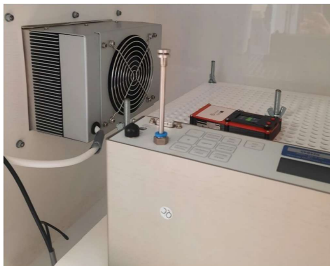
Figure 1. Laboratory assessment of LCS SPS30.
