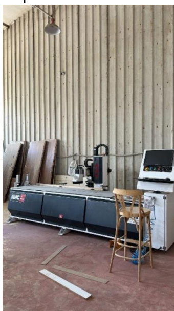
CNC machine for hinges, locks and handles of doors
