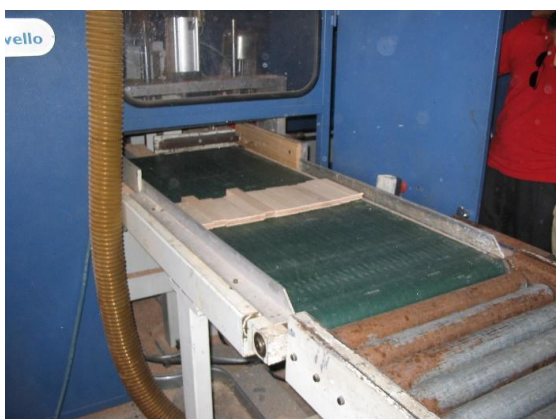
Finger-joint profile machine
