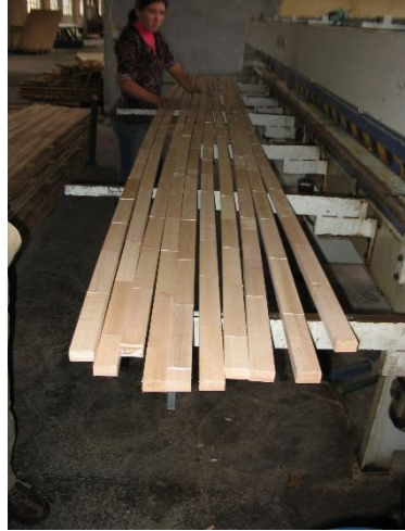
Joined blocks into the strips
