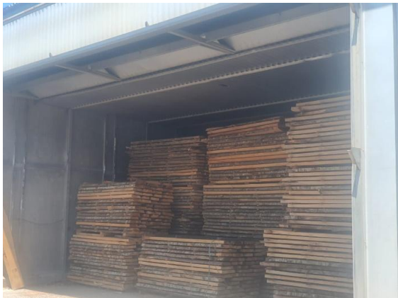
Dried beech boards inside the kiln
