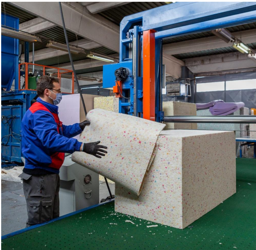
Re-bonded foam block ready for further processing
