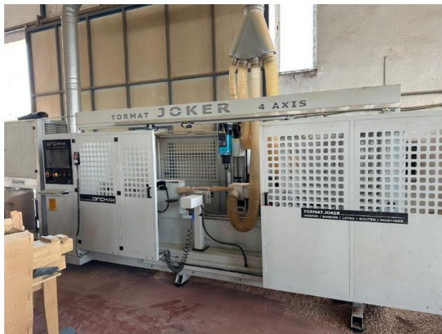
4-axis CNC wood lathe machine
