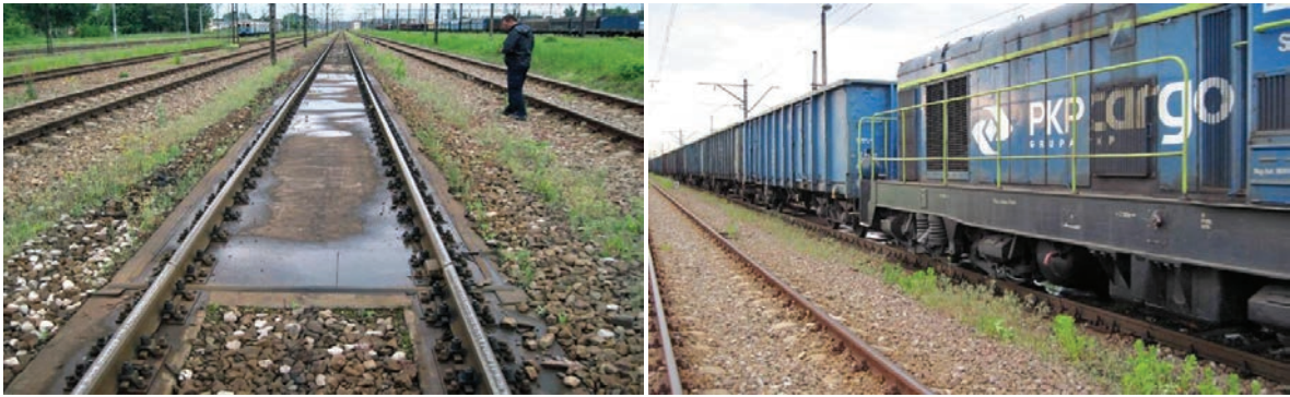
Fig. 6. Low-speed weigh-in-motion system for train weighing (left) and one of the calibration trains on it.
