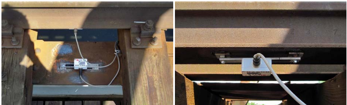
Fig. 3. Strain sensors attached over glued mounting plates.
