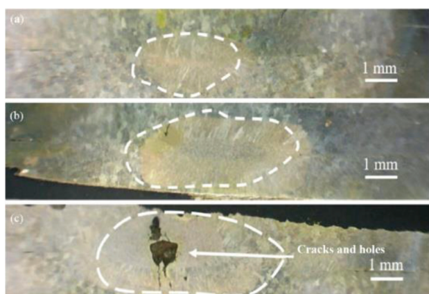
Figure 6: Macroscopic appearance of spot-weld joints
