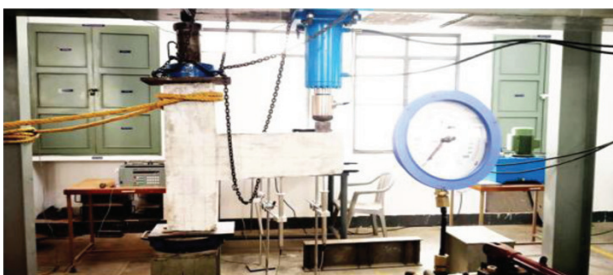
Figure 6: Experimental Setup for Beam – Column Joint
