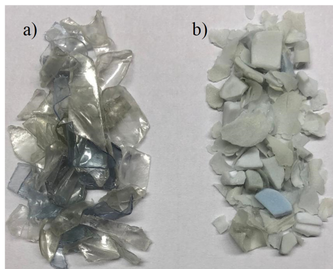
Figure 3. Visual representation of (a) starting PET flakes and (b) PET residues.
