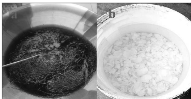
Figure 2: Alkaline treatment of nanoparticles (a. Cocos nucifera fibre & b. Eggshells)
