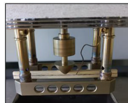
Figure 1: Sample geometry and DMA 3-point bending test specifications.
