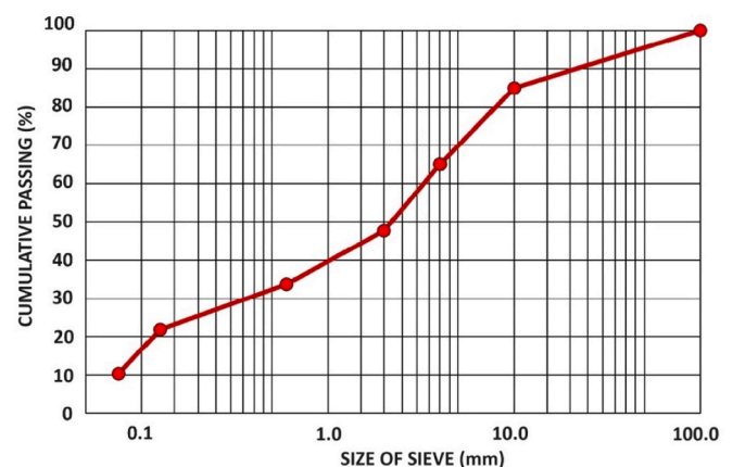
Fig. 1. Gradation curve of the natural aggregate.
