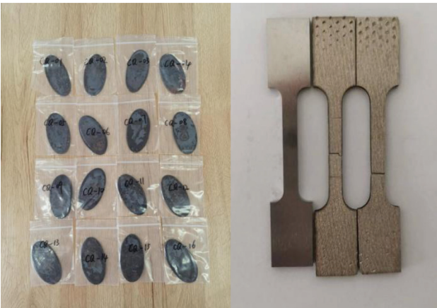
Figure 7: Photos of rolled test plates and tensile test specimens
