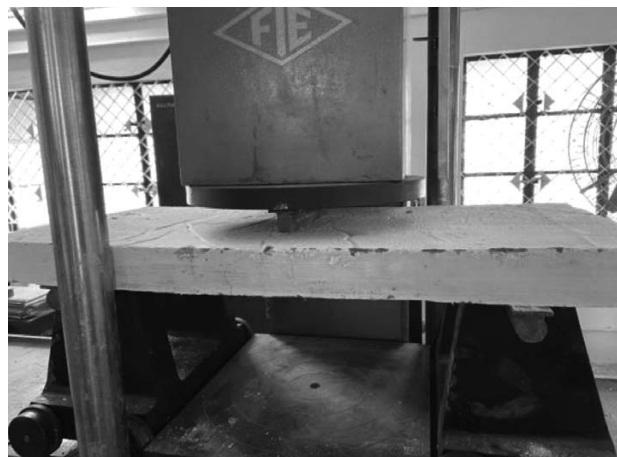
Figure 5: Testing of a fire-damaged slab
