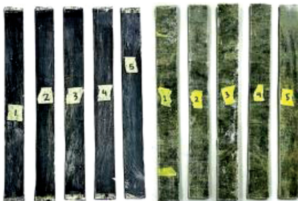
Figure 2: Test specimens: a) abaca/epoxy-bamboo activated carbon nanofiller; b) abaca-E-glass/epoxy-bamboo activated carbon nanofiller
