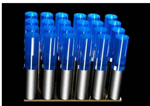
Figure 7. Schematic illustration of Au-PPy nanorods.
