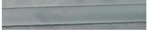
Figure 4: Rotation speed 800 \text{ min}^{-1} , welding speed 300 \text{ mm/min}
