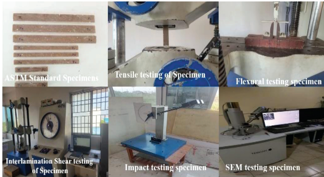
Figure 2: Experimental testing of specimens for glass-fiber hybrid composite with nanoparticles
