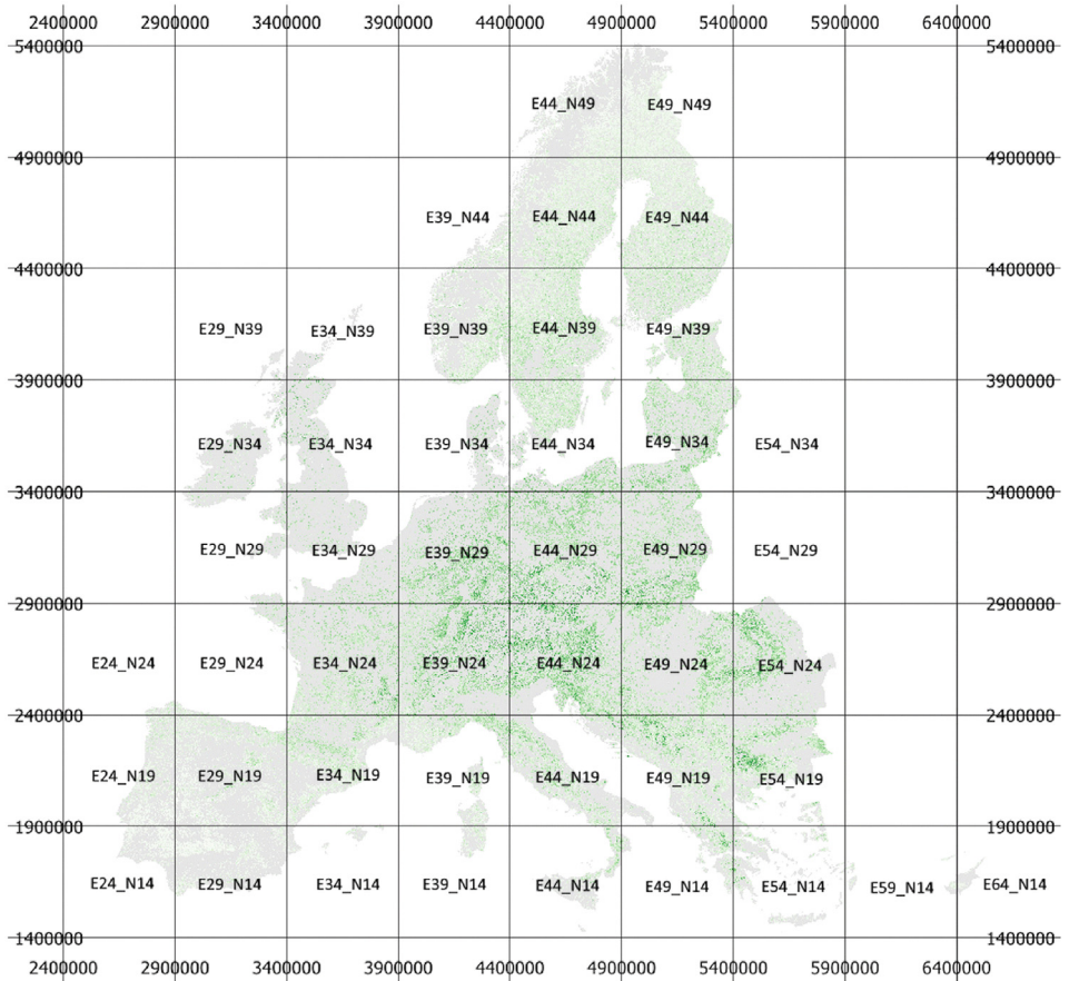
Fig. 2. Maps are provided in 10 m spatial resolution in 500×500 km tiles in the EPSG:3035 - ETRS89-extended / LAEA Europe projection. Volume map as background in the image.
