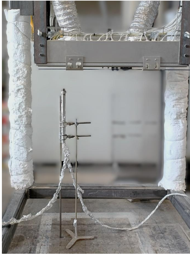
Fig. 4 Heat flux gauge positioning during HIFREP calibration
