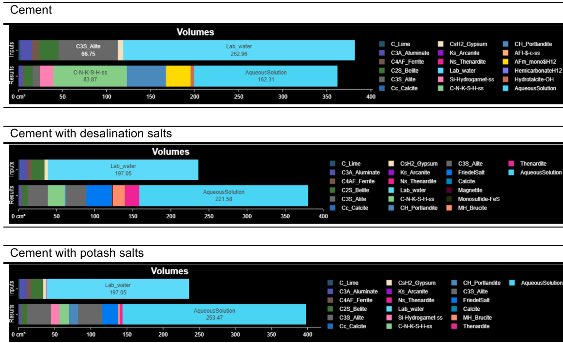
Fig. 12. CenGEMS simulations of three cementitious systems: plain cement, cement with desalination salts and cement with potash salts.
