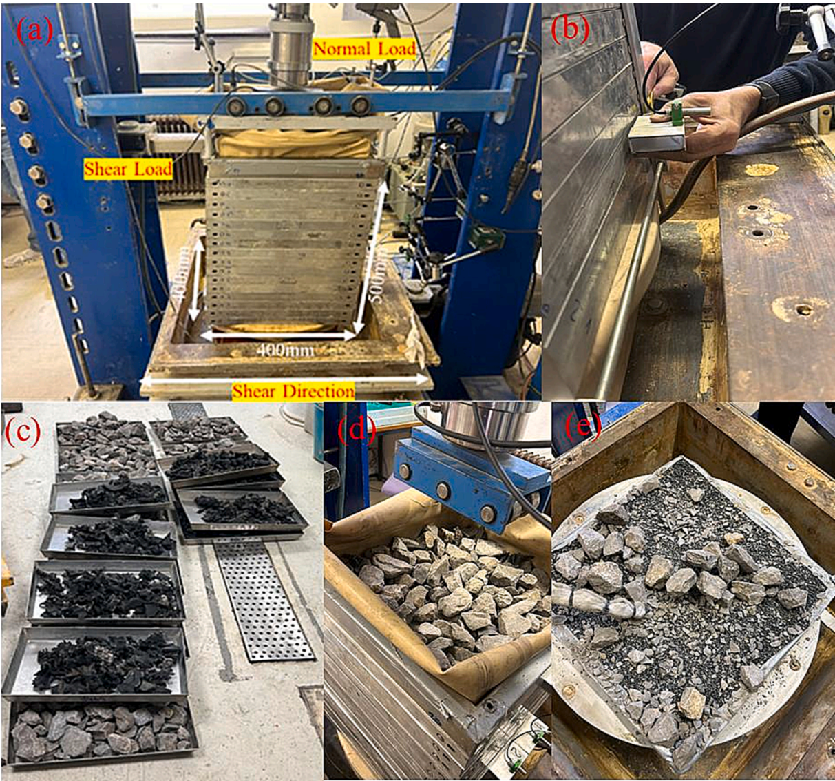
Fig. 4. Pictures of cyclic simple shear test (a) Experimental arrangement (b) Displacement transducer (c) Sample preparation (d) Sample preparation in apparatus (e) Degraded material after the test.
