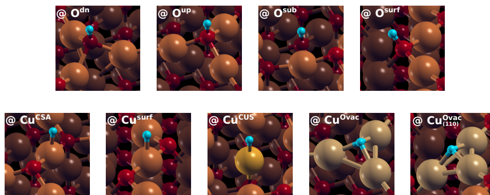
Figure 13. Snapshots of optimized structures of H adsorbed at various O (top row) and Cu (bottom row) sites on \text{Cu}_2\text{O} surfaces. Note that, upon adsorption of H onto \text{O}^{\text{dn}} site, the \text{O}^{\text{dn}} shifts upwards above the plane of surface \text{Cu}^{\text{CSA}} ions; hence, the H @ \text{O}^{\text{dn}} appears visually similar to H @ \text{O}^{\text{up}} .
