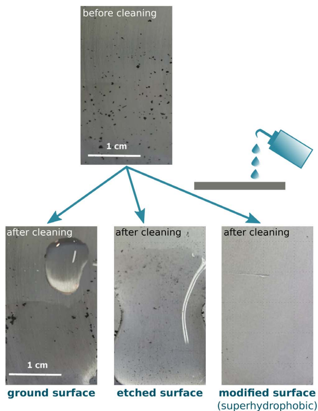
Figure 14. Snapshots recorded before (upper panel) and after (lower panel) cleaning of different surfaces: ground Al, Al etched in 0.1 M NaOH at 90°C, cooled to room temperature and Al etched in 0.1 M NaOH and then immersed in ethanol solution of 5 mM octadecanoic acid (CA-18) for 30 minutes. Carbon particles were used for the self-cleaning test. Video film is presented in Supplementary material (Video information VI-1).
