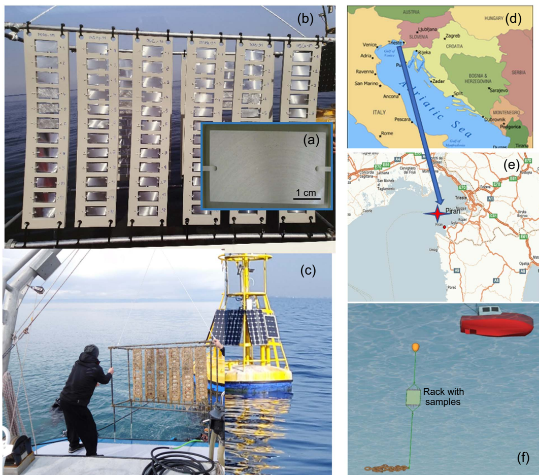
FIGURE 2. (a) Individual sample, (b) frame with racks with samples, (c) removal of the racks with samples from the seawater near the buoy, (d, e) maps of the immersion site (coordinates 45° 32.925' N, 13° 33.042' E), and (f) positioning of the racks with samples at a depth of 20 m.
