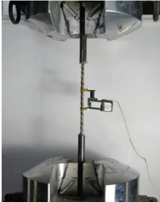
Figure 1: BFRP bar loading in place for tensile test
