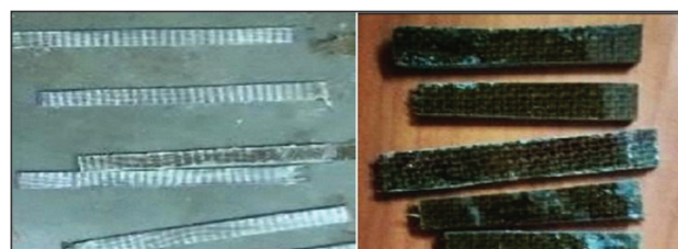
Figure 3: Flexural test specimens before and after the test
