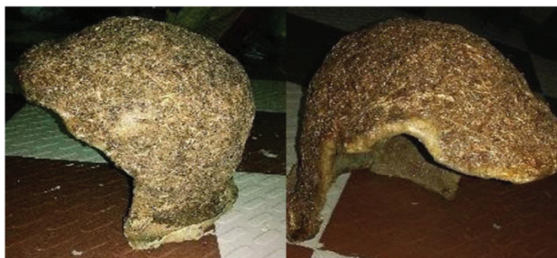
Figure 8: Fabricated model of the helmet made from the hybrid composite
