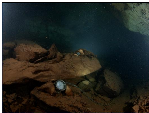
Figure 2. Installation of an IR camera with integral IR lights (top) and an independent stand-alone IR LED emitter array below it (photo: A. Sáři).
