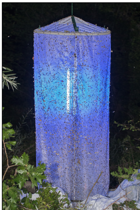
Figure 1. Light trap set at the basecamp Ulog, next to the Neretva River: 180 cm cylinder with two superactinic UV-lights.
