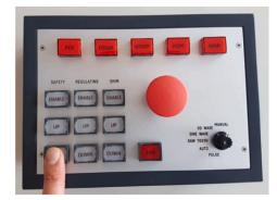
(b) A hardware console was developed for the Research Reactor Simulator.
