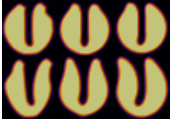
FIG. 15. interRKFoam solver. Left column: algebraic, middle: PLIC, right: MPLIC interface capturing method. Top row: after one rotation, bottom: after five rotations. Mesh size: 100 \times 100 .
