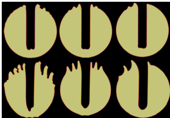
FIG. 16. interRKFoam solver. Left column: algebraic, middle: PLIC, right: MPLIC interface capturing method. Top row: after one rotation, bottom: after five rotations. Mesh size: 500 \times 500 .
