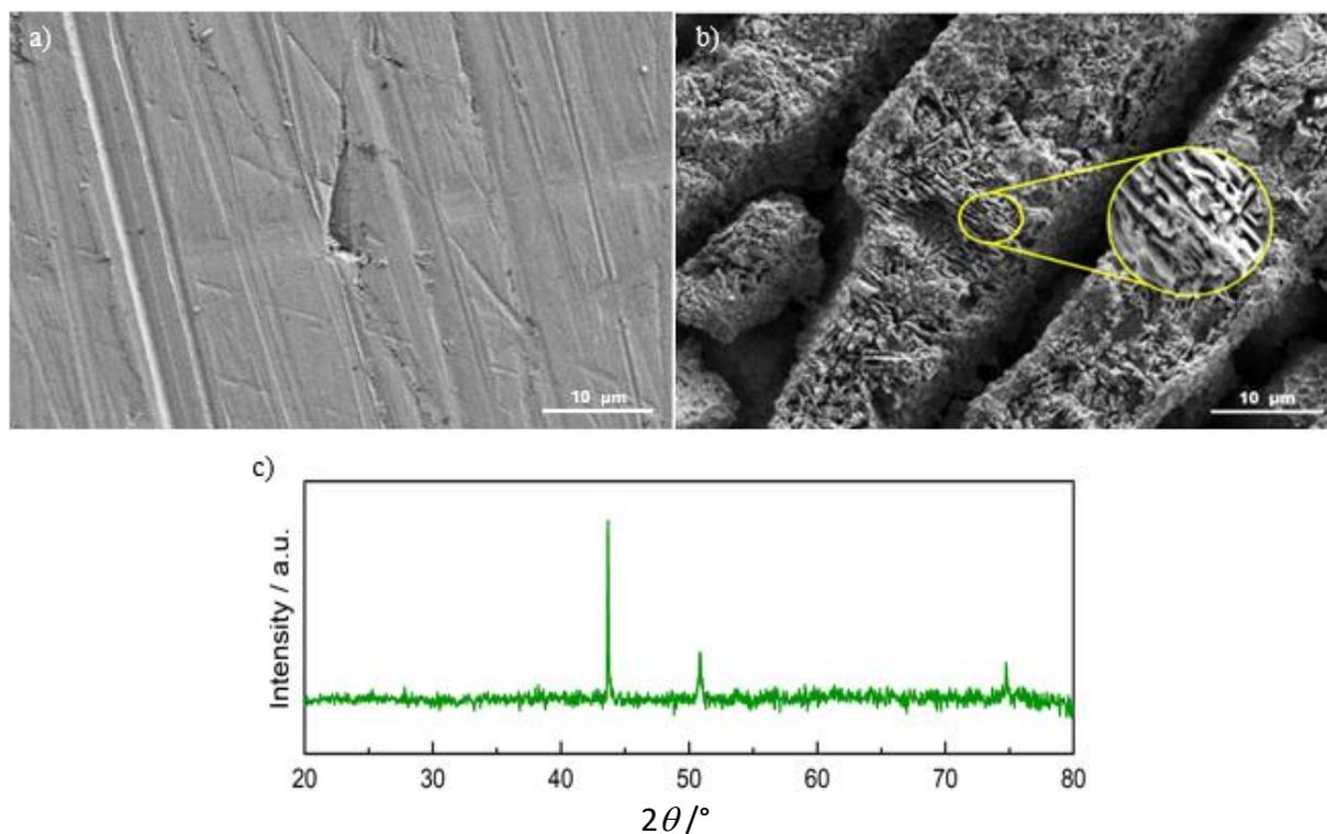
**Figure 1.** SEM micrographs showing: a) the initial alloy used for catalyst preparation, and b) the catalyst prepared with nitridation and anodization of the alloy shown at two magnifications. Inset circle diameter is 7  $\mu\text{m}$ . c) XRD diffractogram of the catalyst showing peaks related to the compositionally complex alloy
