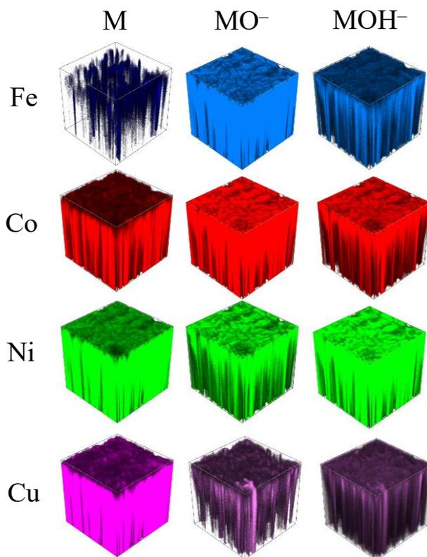
**Figure 3.** 3D ToF-SIMS images showing  $M^-$  ( $M = Ni, Fe, Ni$  or  $Co$ ), and the corresponding signal for  $MO^-$  and  $MOH^-$ . The analysis was performed after the electrocatalytic glycerol oxidation tests
