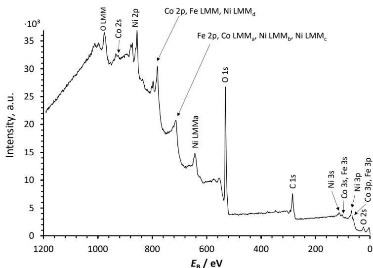
**Figure 2.** The XPS survey spectrum of the sample showing signals for Fe-, Co-, Ni-, C-, and O-containing species. The XPS surface analysis was performed after the electrocatalytic glycerol oxidation tests
