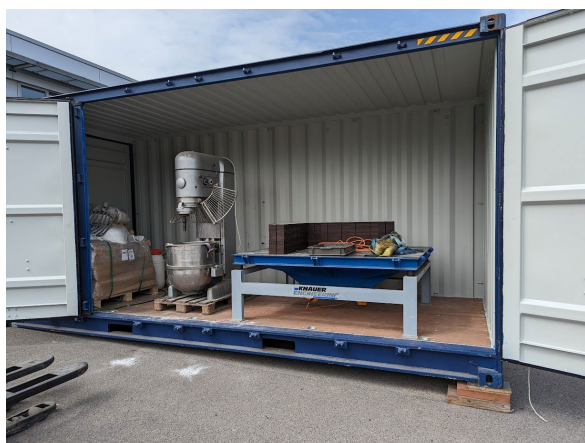
Figure 1: KU Leuven mobile unit for the production of GEORIS pavers
