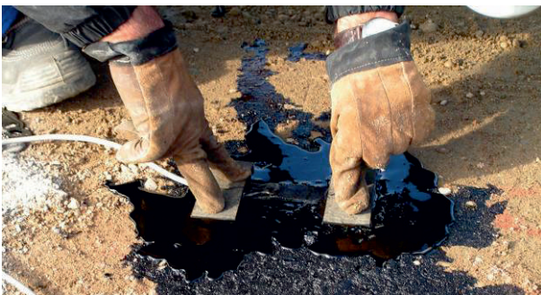
Figure 4. Installation of strain gauge.
