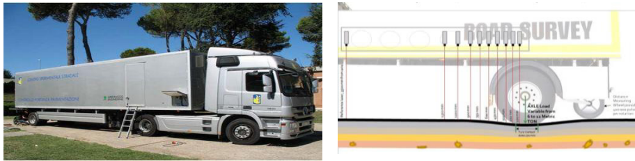
Fig. 2. (a) The TSD (b) schematic of laser layout (South African TSD).
