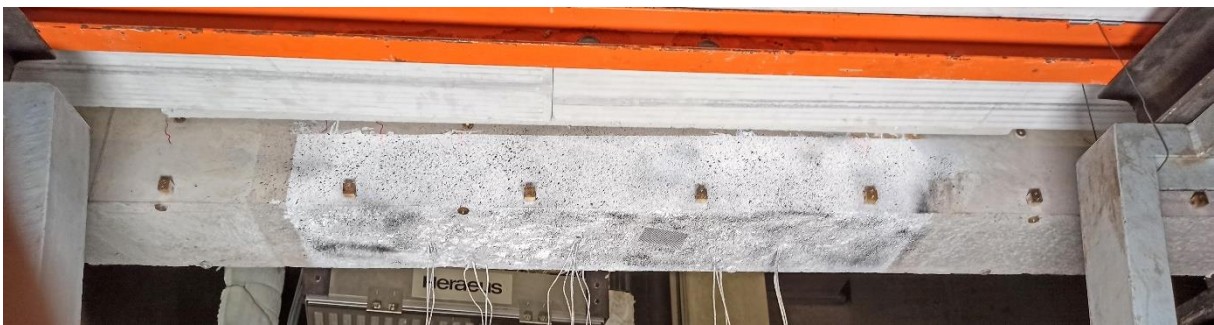
Figure 5. The compressed side of the beams monitored using the Digital Image Correlation (DIC).
