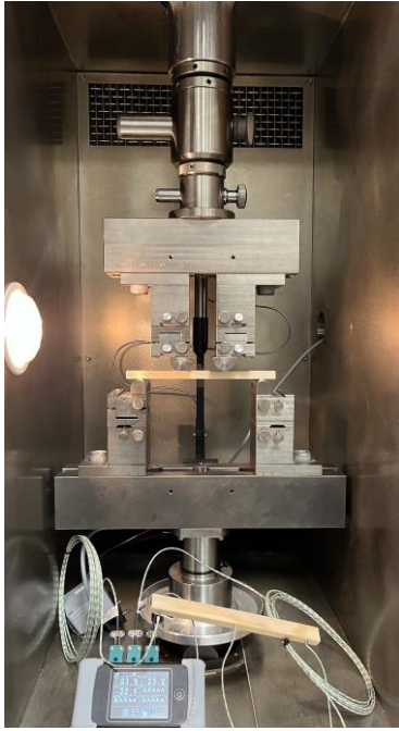
Figure 1. Test setup for four-point bending test at elevated temperature.
