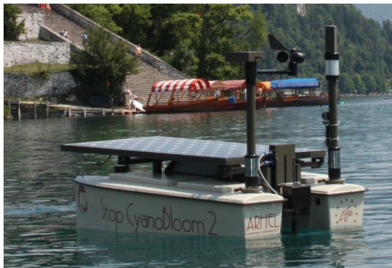
Photo 1: LIFE Stop Cyanobloom robotic vessel in operation on Lake Bled.
