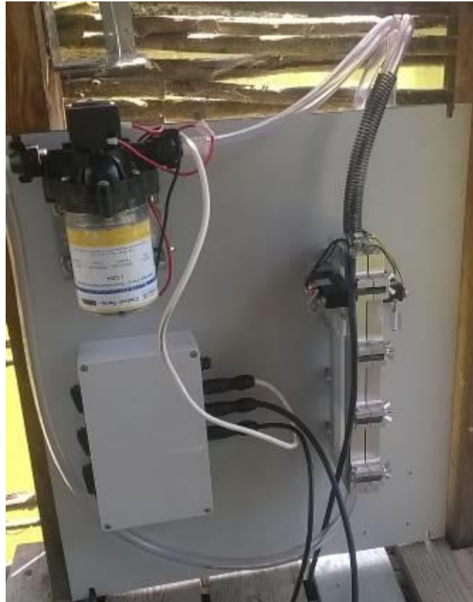
Figure 15: Set-up of the second pilot test experiment on Koseze Pond with electrolytic cell: a system with power supply, pump and an electrolytic cell.
