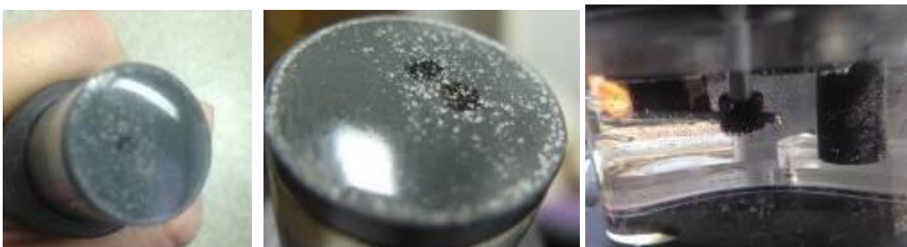
Figure 19: Damages on the epoxy surface of the fluorescence sensors and emerging of the bubbles in the measuring chamber, both causing a false reading of the produced fluorescence signals.
