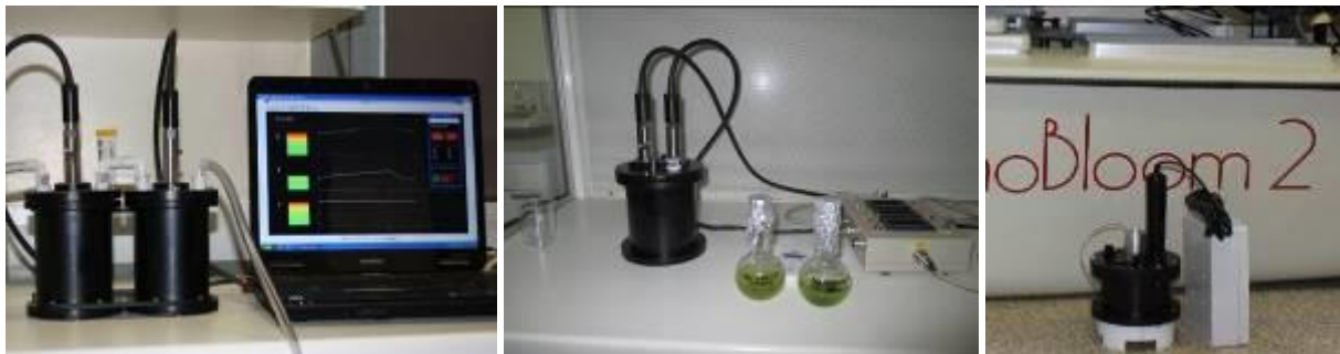
Figure 5: Laboratory calibration of the phycocyanin and chlorophyll sensors in measuring chamber. In the course of the laboratory tastings, a transfer from double (left) to single measuring chamber equipped with two fluorescence sensors (middle) has been made. The right picture shows measuring chamber with electronics prepared for integration into the vessel.
