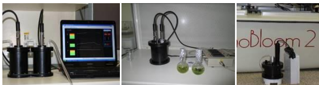
Figure 5: Laboratory calibration of the phycocyanin and chlorophyll sensors in measuring chamber. In the course of the laboratory tastings, a transfer from double (left) to single measuring chamber equipped with two fluorescence sensors (middle) has been made. The right picture shows measuring chamber with electronics prepared for integration into the vessel.
