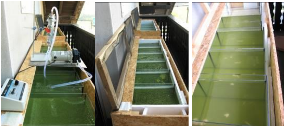
Slika 1: Set-up of the electro-oxidation cell for water treatment and pump along the aquariums with the water taken from a fish pond in Hotinja Vas.
