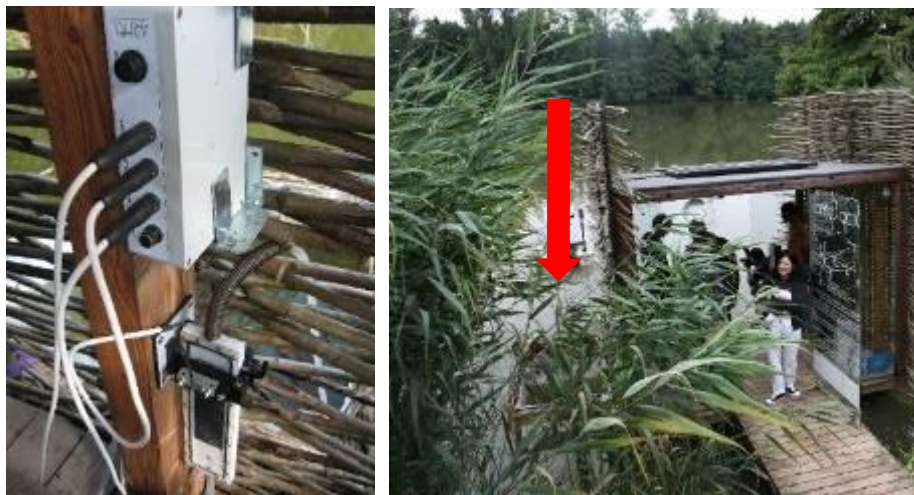
Figure 14: Fixed electrolytic cell in the inner side of the service wharf and location of the experimental canisters
