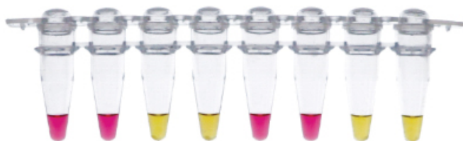
Figure A6. Colour of negative and positive reactions. Negative reactions will remain pink and positive reactions will turn yellow (can also be orange in case of a weak reaction).
