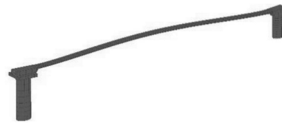
1 st FE model mode shape: f_2 = 0.70 Hz
