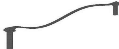
2 nd FE model mode shape: f_3 = 1.09 Hz
