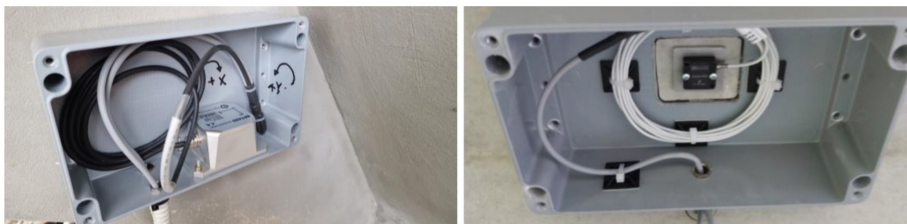
Figure 5. Sensors used for the permanent monitoring: biaxial inclinometer (left) and uniaxial accelerometer (right).
