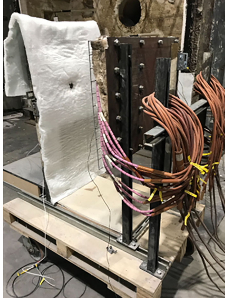
Figure 14. Photography of the measurement of the incident heat flux with a thermal shield (ceramic fibre) around the heat flux gauge.
