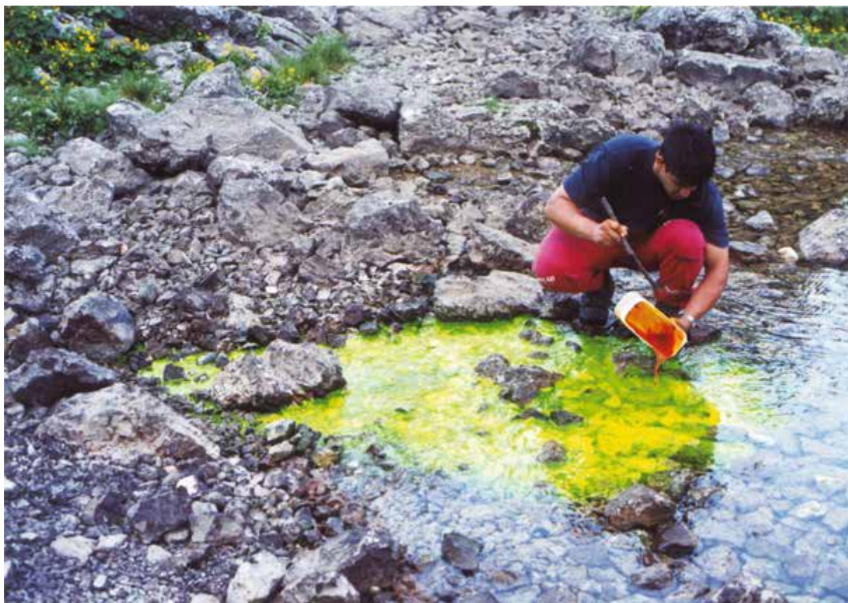
Injiciranje fluorescentnega sledila uranin v ponor (Foto: Janko Urbanc) Injection of fluorescent tracer uranine into the Močivec sinkhole (Photo: Janko Urbanc)
