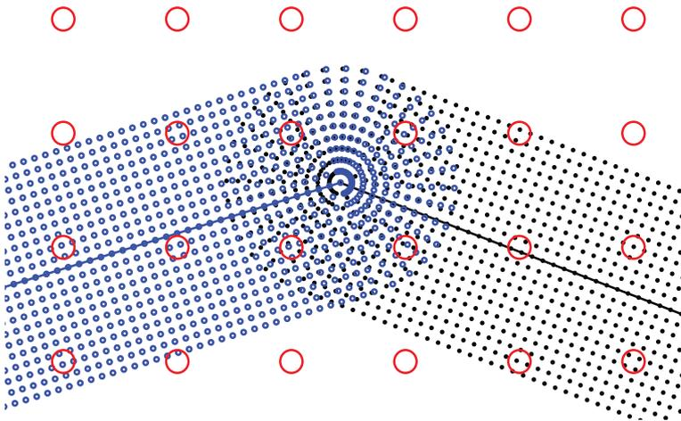
**FIGURE 1.** Points in 1m grid for two spans of a power line are shown with blue and black dots in which the program determined the values of the extremely low-frequency (ELF) magnetic fields (MF). Red circles represent the final 10 mgrid for which the final results were generated.
