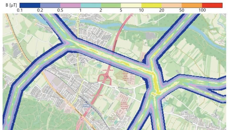
**FIGURE 4.** Example of the total value of the extremely low-frequency (ELF) magnetic fields (MF) of several high voltage power lines around distribution transformer stations for nominal load in the area of the capital city of Ljubljana (approximately 5 x 2.7 km).
