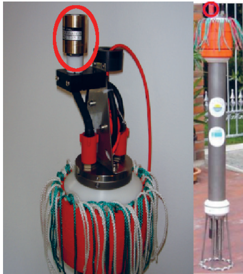
Figure 3. PAR sensor ( left ; circled with a red line) on top of a microstructure probe ( right ).
