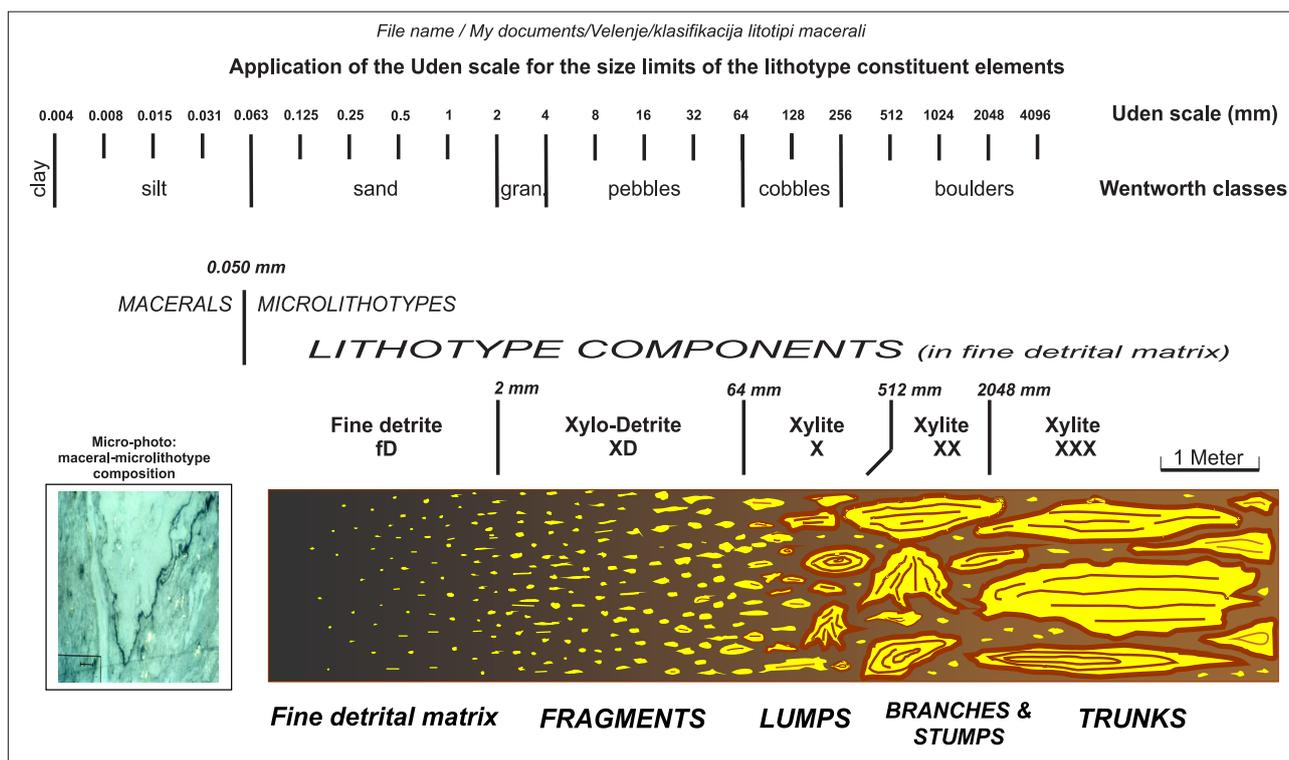
Fig. 9. Basic concept of macropetrographic classification for the Velenje ortho-lignite (Markič et al., 2001; Markič & Sachsenhofer, 2010) using a concept of lithotype components and the Uden scale for dimension limits.
