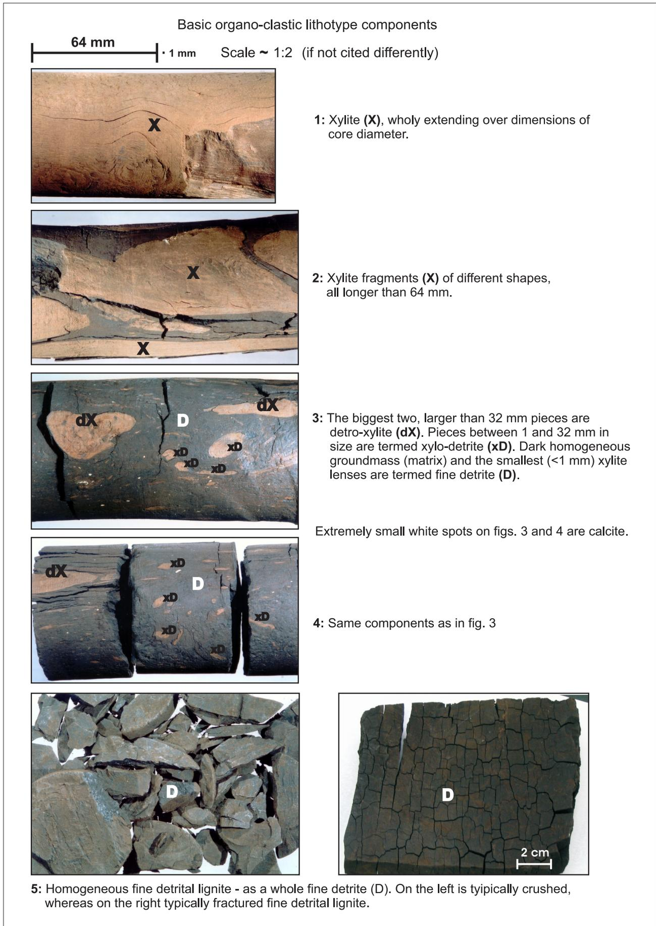
Fig. 10. Lithotype classification is employed in macro-petrographic core logging of the Velenje ortho-lignite. JGM-55 borehole (excavation field B k.-130) (this study) (see appendix) is an example of petrographic well-logging.
