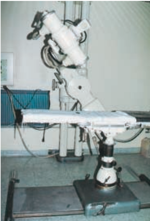
Figure 3. Stabilipan, a 300 kV device for radiotherapy, suitable for superficial irradiation, and allowing 3 to 5 combinations of voltage, made by Siemens.
