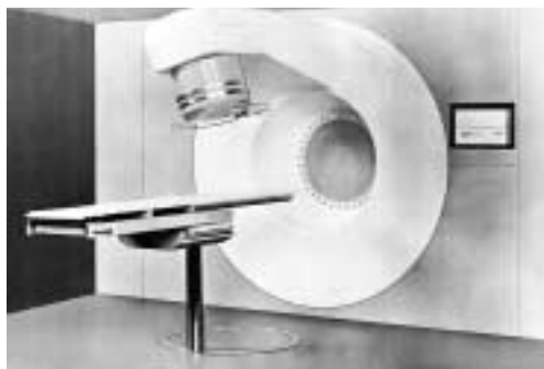
Figure 16. The linear accelerator SL75/20, a supervoltage radiotherapy device made by Phillips . It was used until the year 2000.
