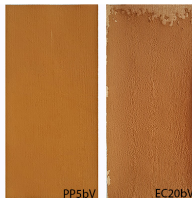
Figure 2: Photograph of samples, printed with printing paste Printperfekt Lac 110 Neu (5 wt.% of pigment) – PP5bV, and Elastil Coprente FG (20 wt.% of pigment) – EC20bV, showing the differences in colour and quality of the print
