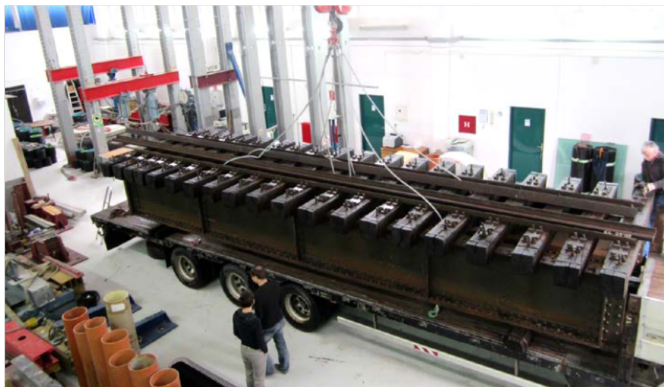
Figure 2: Original Buna bridge transported to the laboratory before testing [12, 13]
