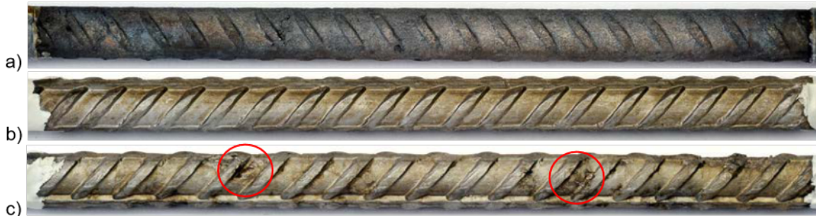
Figure 6: Corrosion damages on steel bar embedded in a) FA8, b) S3a-661 and c) MK2 mortar after 17 cycles of exposure.
